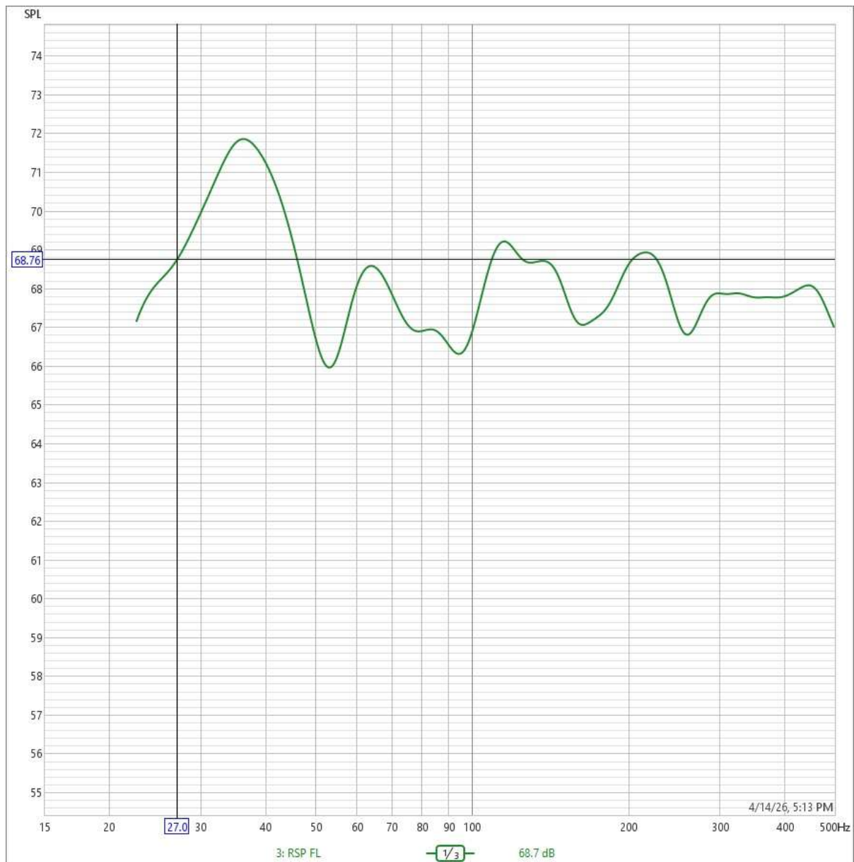
Bass Response (not Spatially Averaged), Front Left Channel
