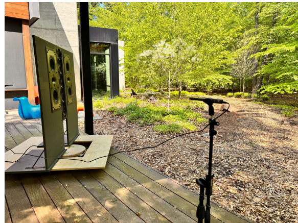
Sonance R2 Horizontal Response Testing
