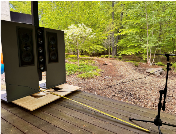
Sonance R2 Speaker Measurements (UMIK-1 @2m)
