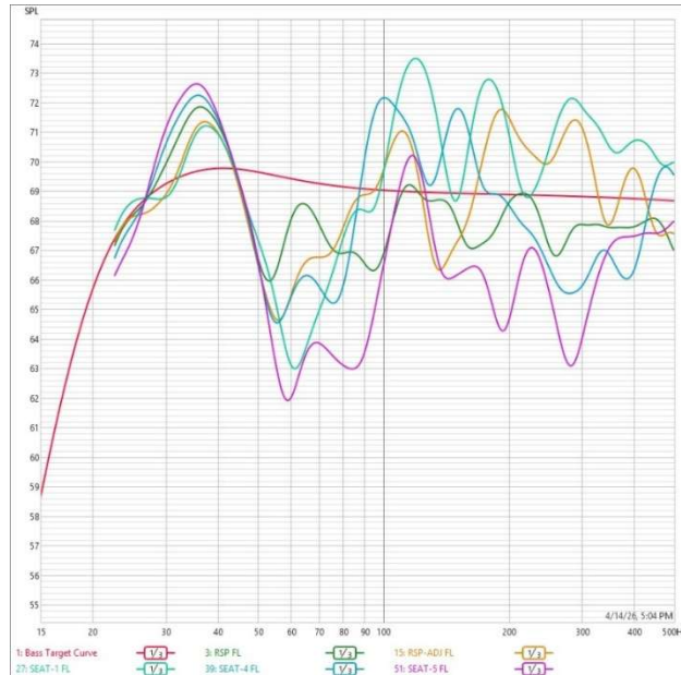
Frequency Response Normalized to Target Curve (not Spatially Averaged)
